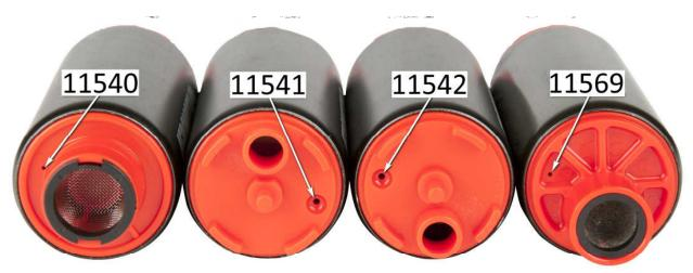
Please note the location of the vapor-purge port for your model Stealth 340, as illustrated above. During installation, be certain to check for and eliminate any blockage or restrictions to this port. Failure to do so may result in slow or no priming and may damage your 340 pump due to dry run.
